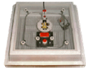
Incubator with manual thermostat.
